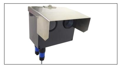
The TDC3 Series are advanced traffic detectors using Doppler Radar, Ultrasound and Passive Infrared technology. TDC3-2-F models provide comprehensive traffic data including individual vehicle class (by vehicle length), per vehicle speed, occupancy time and time gap.
