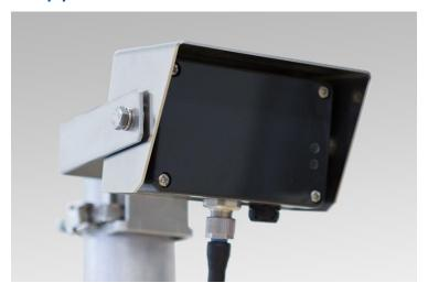
The TDD1-MW series of traffic detectors uses microwave Doppler radar technology for detecting vehicles moving through its field of view. For the duration of the detection, a contact closure relay output is activated. When the detection ends, the contact is released into its normal state. The factory-set configuration can easily be altered using an IR remote control (extra accessory).
