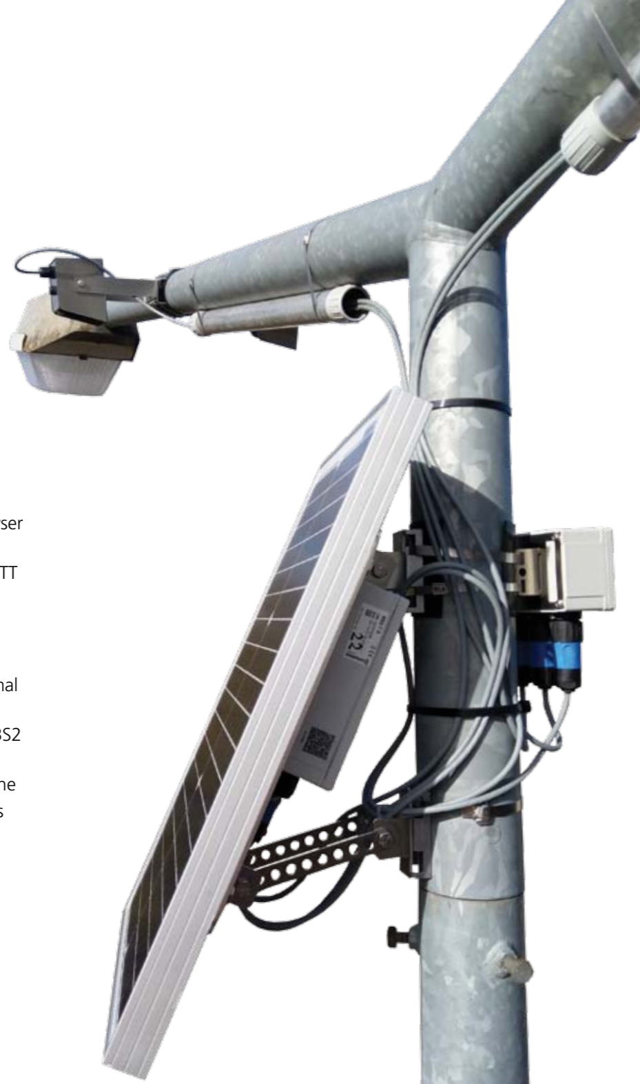
BS2-TS30 with four TDC1-PIR and JBL3 junction box in Regensburg (Germany)
